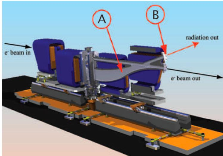
**Figure 1.** Rendering of the UCLA-built ATF chicane compressor Cutaway view shows the radiation source region between the third and fourth dipoles (A) and the radiation extraction port (B).
