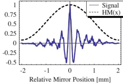
**Figure 5.** (left) Autocorrelation of CER using Michelson interferometer and cryogenic bolometer, along with Hamming window function for apodizing FFT.
