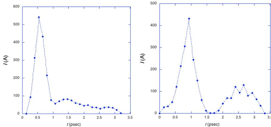
**Figure 3.** Reconstructed longitudinal beam profiles using Kramers-Kronig analysis of CTR: (left) optimum compression, (right) over compression.
