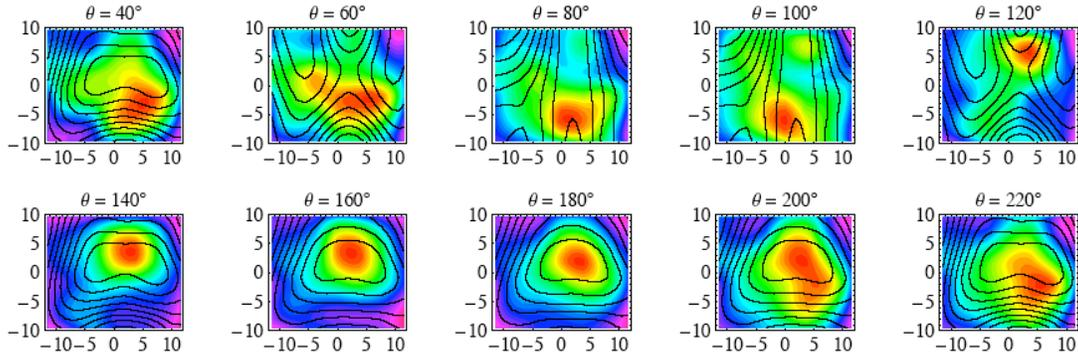
**Figure 7.** CER far-field angular distributions as a function of polarizer angle in UCLA/ATF compressor, taken under maximum compression conditions.
