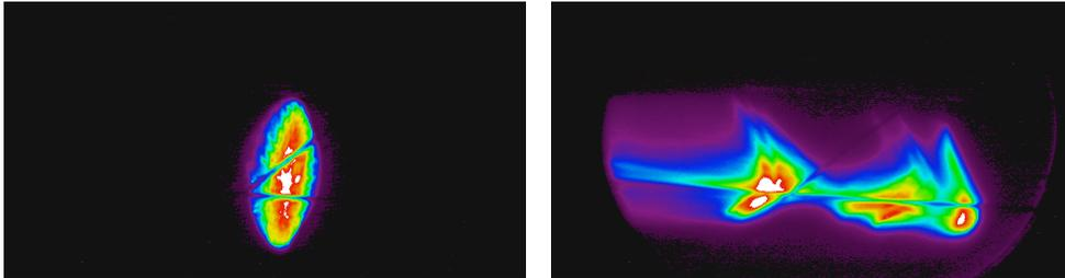
**Figure 2.** Beam images in the spectrometer, (bend plane is horizontal): (left)  $9^\circ$  forward of RF crest near minimum energy spread, no compression, (right)  $19^\circ$  forward of crest, maximum compression.
