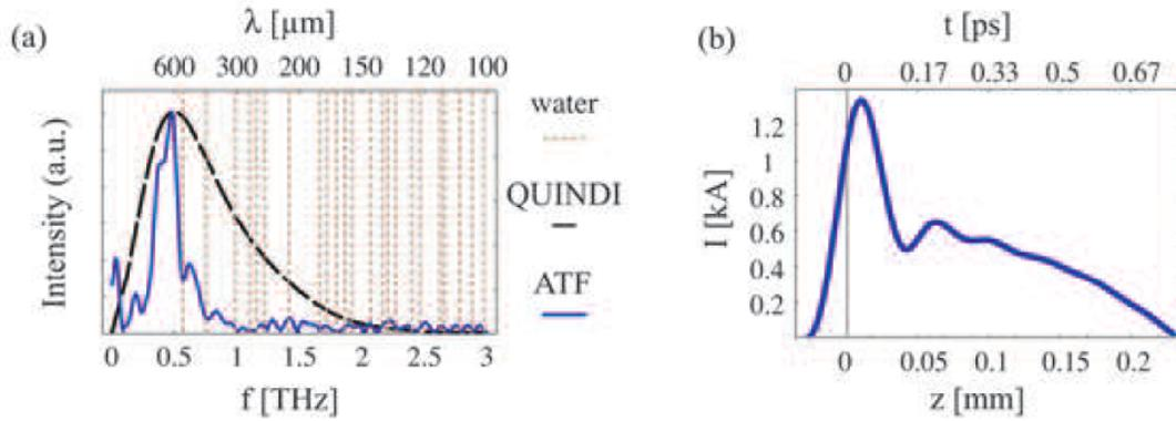
**Figure 6.** (a) Spectra from apodized interferogram and from QUINDI simulation. Prominent water absorption frequencies are shown as vertical dotted lines. (b) Minimal phase Kramers-Kronig bunch reconstruction for the measured spectrum.
