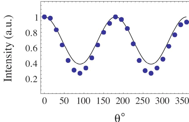
**Figure 4.** Polarization scan of CER at UCLA/ATF compressor, taken under maximum compression conditions. Solid line is the prediction of QUINDI.
