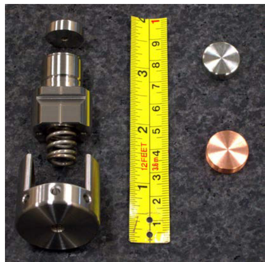
Figure 2: Reusable cathode holder with molybdenum cathode substrate on the LEFT, based on Fermilab's A0 gun. Two undeposited cathodes (stainless steel and copper) on the RIGHT.
