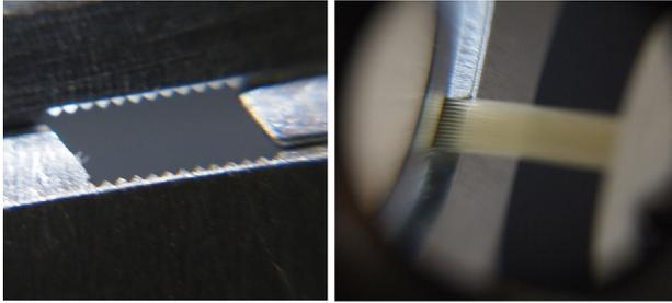
Figure 2: Photograph of fiber array. Fibers are clamped with v-grooves (Left). Fibers Assembled to holder (Right).
