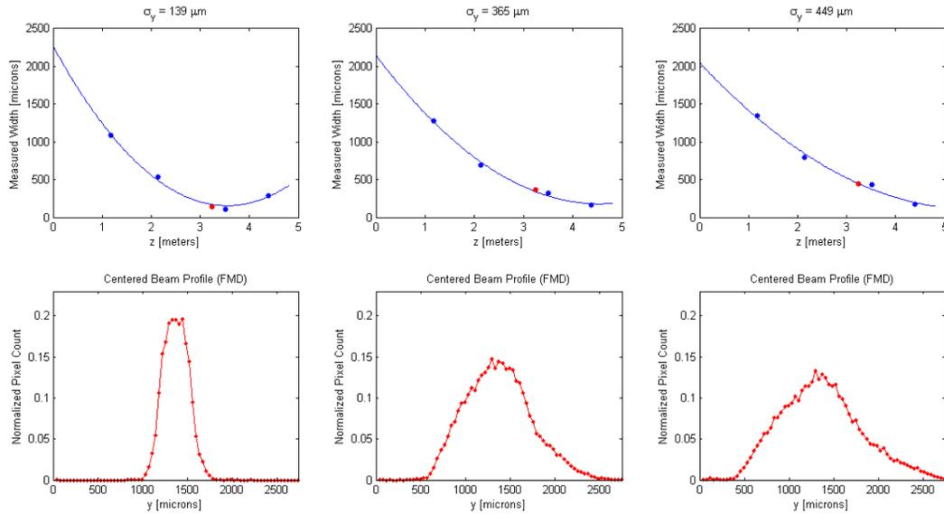
Figure 6: Top Row –Beam widths measured with YAG screens along the beamline (blue). Beam width measured with FMD plotted at the measured z- distance (red). Bottom Row – The averaged beam profile as measured with FMD.
