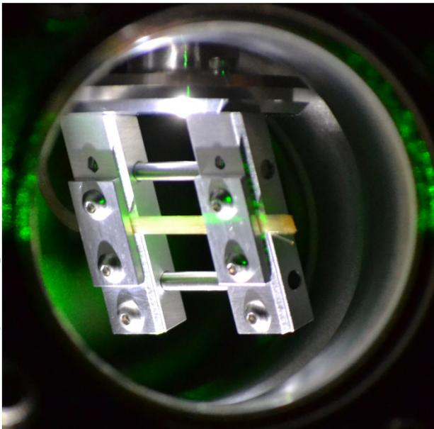
Figure 4: Fiber holder assembly in situ.
