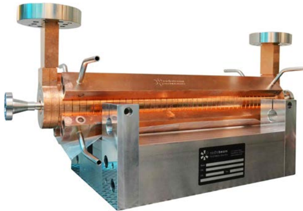
Figure 6: Picture of the XTD deflector after the final brazing and before installation.
