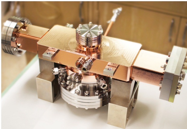
Figure 2: A RadiaBeam-developed photoinjector for the gamma ray ICS system at the STAR facility in Italy.
