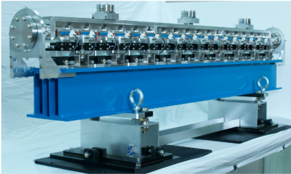
Figure 2: The fully assembled IOTA insert.
