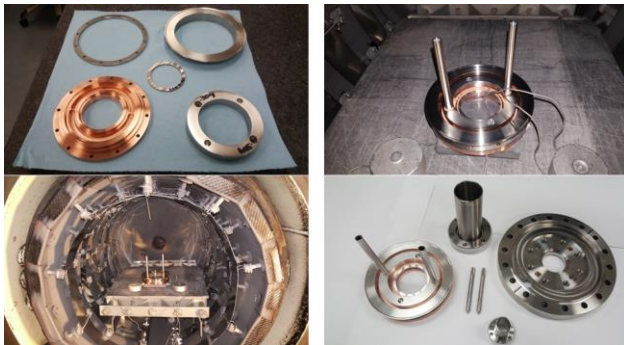
Figure 4: Various parts manufactured and brazed including cooling assembly piece parts (upper left), cooling assembly braze setup in the oven (upper right and lower left) and parts sent to welded bellows manufacturing vendor (lower right).
