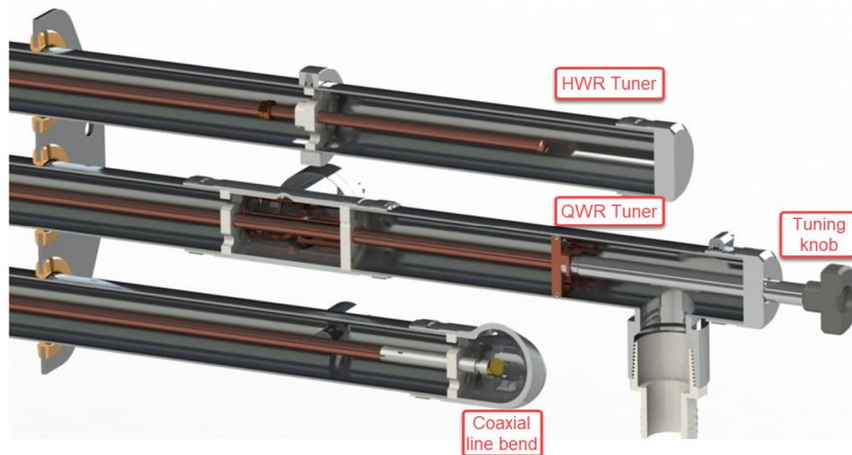
Fig. 16. HWR and QWR coarse tuning mechanisms.
