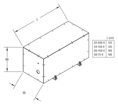
The linac may also be housed in a separate enclosure. Contact RadiaBeam Systems for more information.
