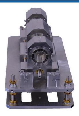
Vacuum-compatible, kinematically-adjustable lattices *(shown above)* are useful for variable source and exit parameters. Each PMQ can be longitudinally adjusted with <5 µm resolution and the entire lattice can be adjusted in up to six degrees of freedom. Optional motorization is available for the utmost versatility.
